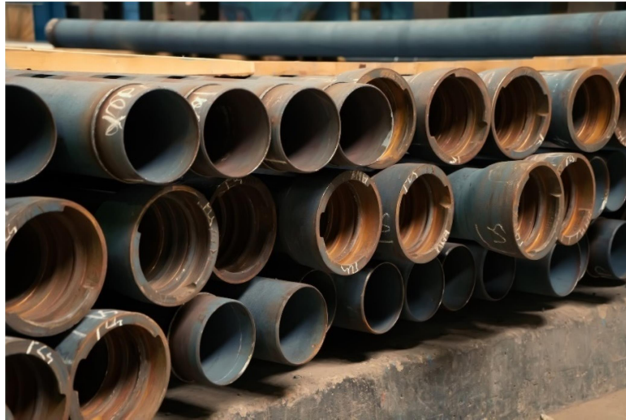
FIGURE:- CAST IRON PIPES
